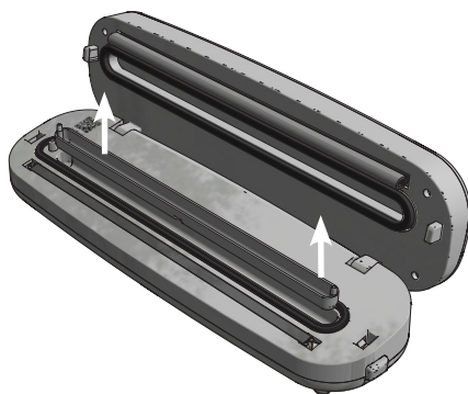
Figure 5: When liquid finds its way into the vacuum channel, lift the Liquid Trap tray directly upwards, pour the liquid out, wash and dry the tray thoroughly.
